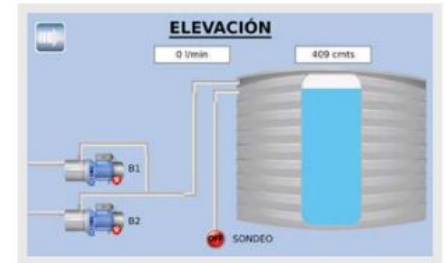
Another overview page shows both pumps are currently deactivated.
